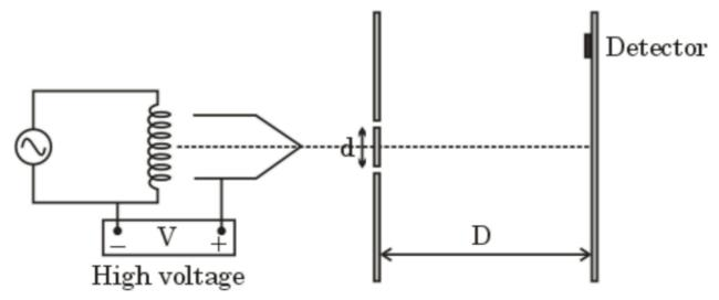
A. the wavelength of electrons after it comes out of the gun is  $\frac{h}{\sqrt{2meV}}$
